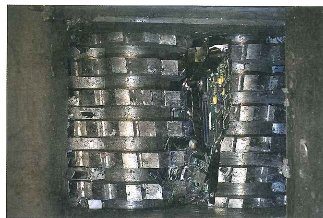
Figure 16-4. This machine is crushing and shredding a hard drive, which will completely destroy the data on the drive.
